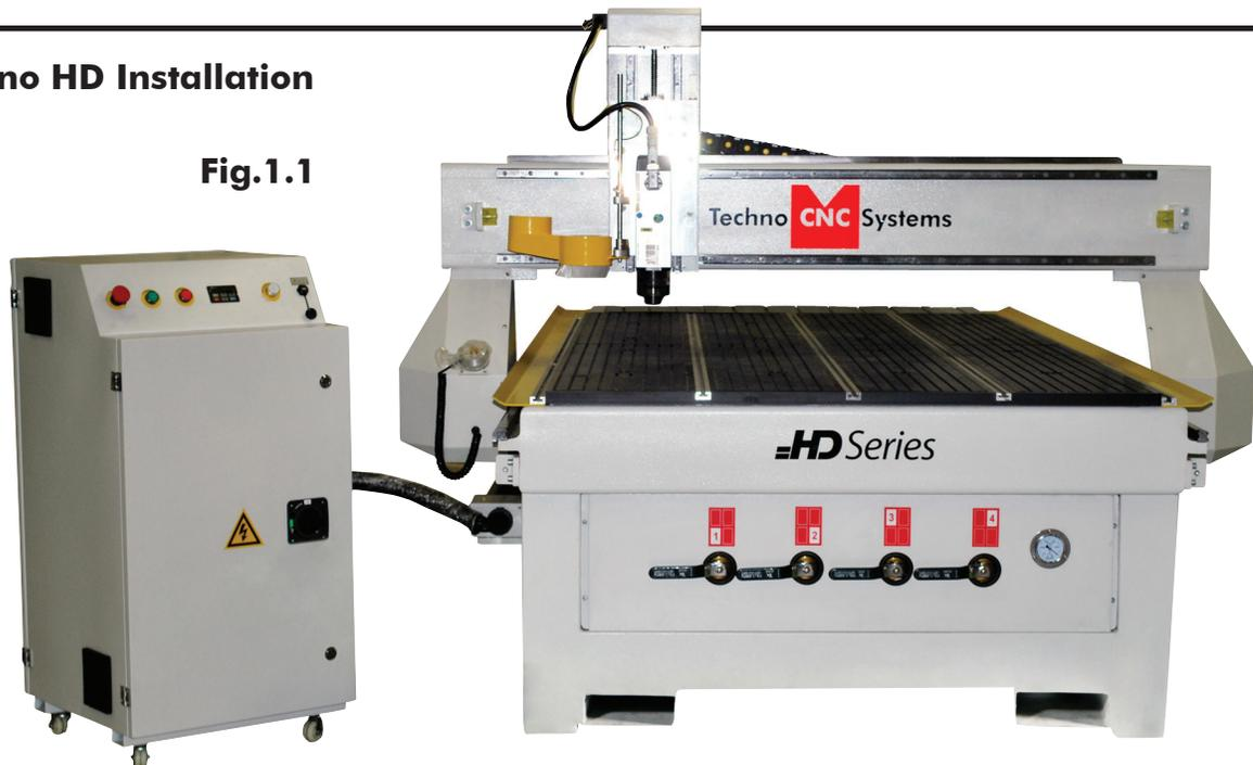
Carefully remove the HD from its wood pallet. Be sure to remove the brackets from its four feet as well as anything stowed under the HD during shipping.
